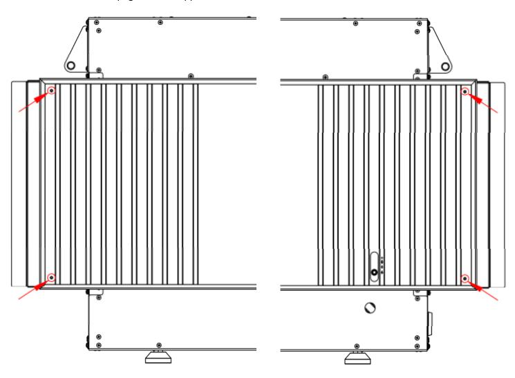
Data plate location—record serial number prior to fitting the trim.
