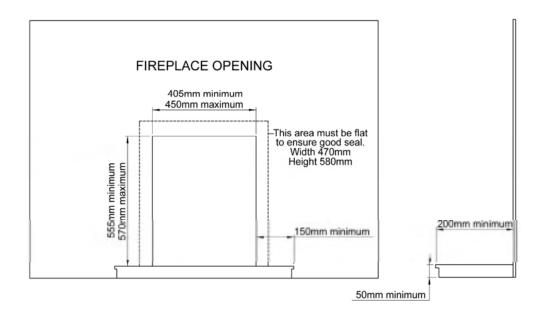
A flat face of a minimum 470mm wide and 590mm high must be provided around the fireplace opening to ensure a good seal is formed. In addition it is important to ensure that the base of the fireplace opening is flat and level with the hearth surface to ensure a secure and aligned installation of the appliance.
