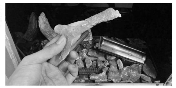
Place log E on the burner tray base at the back of the fire as shown in this picture.
