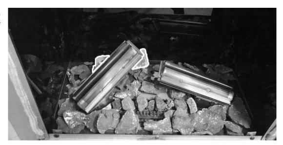
Identify and remove Log D from the ceramic packing carton. Note its orientation for installation in this picture.
