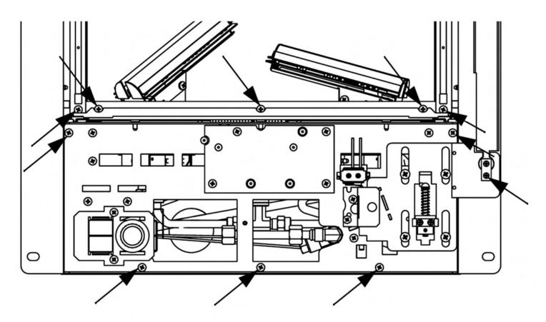
Now carefully pull the burner tray from the fire box. The burner tray is can now be serivced or repaired accordingly—see the following pages for information about removing and replacing serviceable components.
