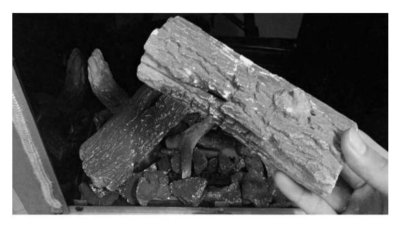
Place log B on the burner tray base at the back of the fire as shown in this picture.
