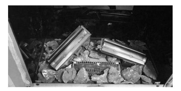
Place the volcanic rock on top of the centre burner as shown. Ensure a 1-2 mm gap is left between each piece. Then using **quarter** of the glowing ember wire supplied, ruffle between fingers to make it loose, about 20mm wide and as long enough to cover the volcanic rock then align over the rock as shown. Ensure no wire is placed within 25mm of the pilot assembly. Retain the rest of the wire for replacement at annual service.
