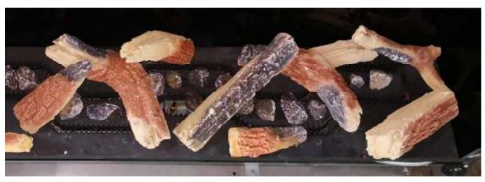
Place the ceramic bark around the ash pan base as shown below. Take care not to place any bark around the pilot burner assembly. Leave at least 5mm from any part of the pilot.
