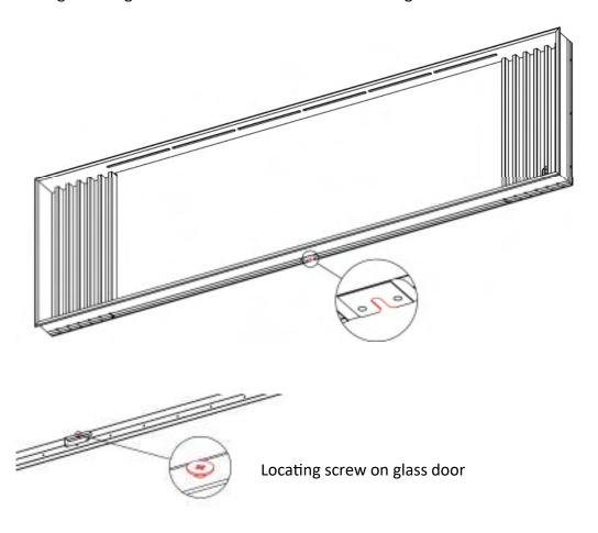
Using the Allen key tool (supplied), tighten the four corner, self locating screws.
