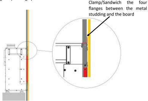
Note: The four flanges sit in front of the metal studding, these will be clamped between the studding and the board.
