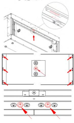
Trim Installation 3.5.2 Once the non-combustible board has been fixed to the studding, the trim can now be fitted to complete the installation.
