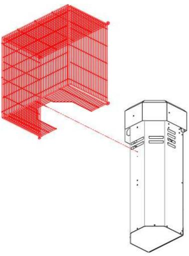
Note: If required, a second basket can be installed in lower position using the prong to locate in the lower hole (drilled to 3mm diameter). This is not a requirement but is available as an additional option.
