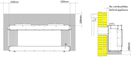
It is recommended that a space of 10mm is left between the back of the appliance and wall. If this is not possible, it is recommended that the plasterboard in this area be removed to provide this clearance.
