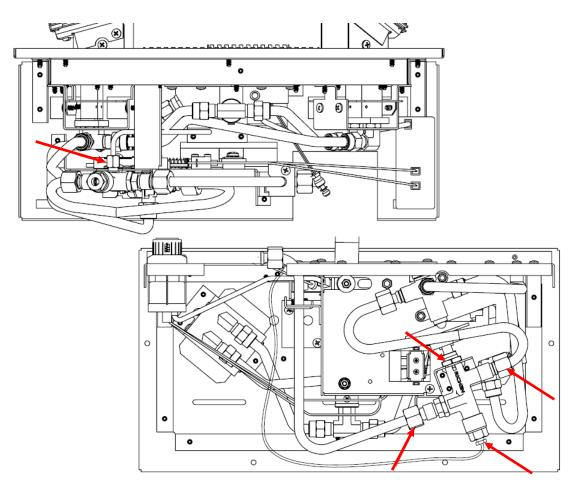
Remove the lock nut to release the valve.
