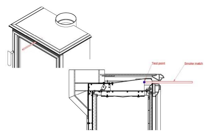
If the appliance fails the spillage test it may be necessary to install a 5" flue liner for the full length of the flue (if not already fitted). If the unit continues to fail this test, turn off the appliance and seek expert advise to expert advice.
