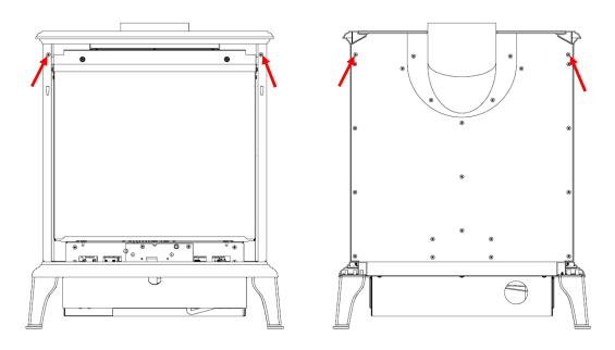
**Step 2.** Remove the four screws as shown
