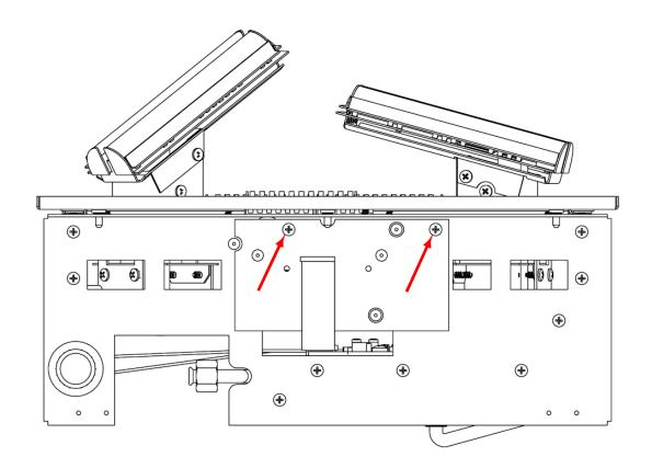
Now remove the HT lead from the base of the spark electrode and remove the two screws to release the pilot. Unscrew the gas inlet nut as shown in the diagram below.
