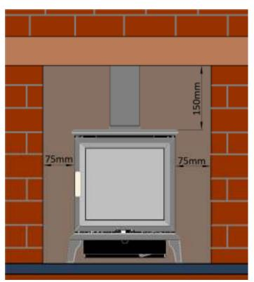
For example, shelf projection = 100mm Clearance must be 175mm (to the shelfs nearest point).
